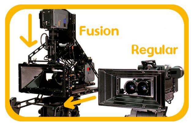
On the right you can see a basic rig. 2 cameras with lenses very close together. On the left is the Fusion rig. The 2 cameras are perpendicular to each other. One looking straight on. And one is from an angle of 90 degrees. Recording a reflection. In the middle there is the most important peace. A special mirror that reflects exactly 50% of the light into one camera. And passes through the other 50% of the light for the second camera.
